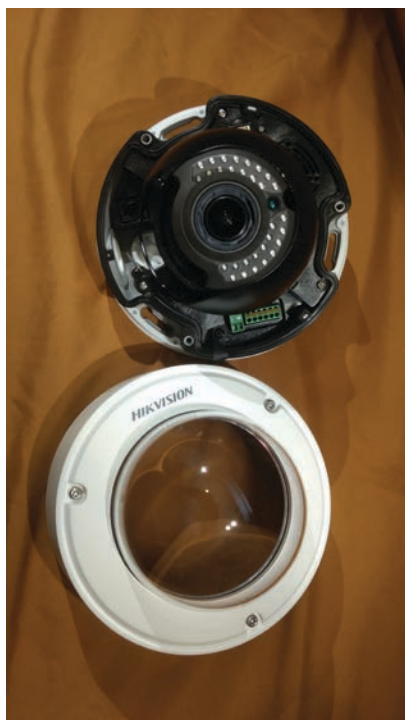
The camera body and external shell have a rubber seal that provides protection from outside elements when the two are mated (left). The device's daytime image (above right) was sharp but its IRs reflected in low light.
