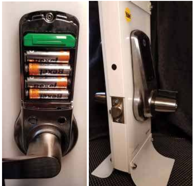
The nexTouch’s plug-in modules (left, above batteries) make adding functionality to the base lock simple. A magnetic door position switch above the latchbolt (right) disables privacy mode when the door is opened.
