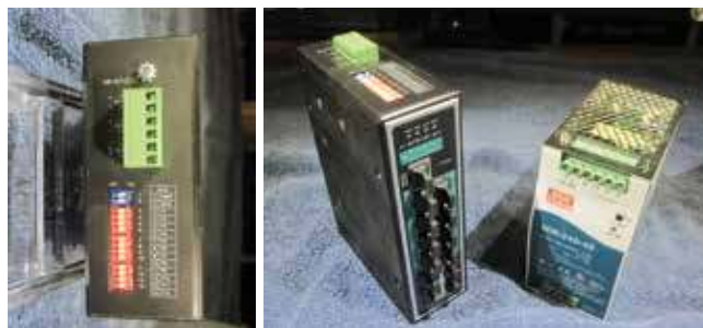
DIP switch configuration of the TI-PG1284i’s alarm outputs (left) makes setting up failure notification a breeze. The separate power supply (right) allows for redundant power where needed.
