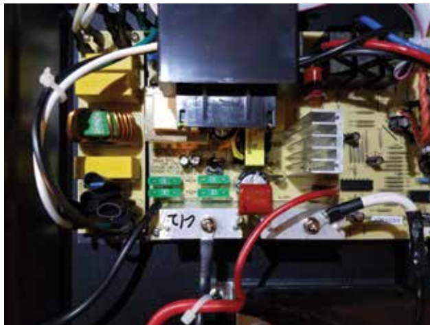
The PRO1500RT’s internal components are protected with heat-shrink tubing rather than common electrical tape, and replaceable automotive-style 30A fuses ensure the value of components protecting the circuit will never change, albeit at the expense of changing a fuse in a failure.
