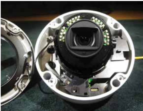
The SNC-VM772R camera has a half moon of IR illuminators built in to its housing, and a rubbery lens protector/shroud to block out the majority of IR “blow-back.” The camera provided a detailed image (right) when set up in an outdoor test environment with vibrant colors and clarity throughout the image field.
