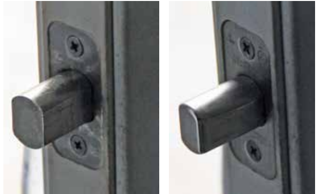
A standard deadbolt (left) can have sharp edges hang up in the doorframe hardware. The tapered face on the Kwikset (right) helps guide the door into the proper locking position.
