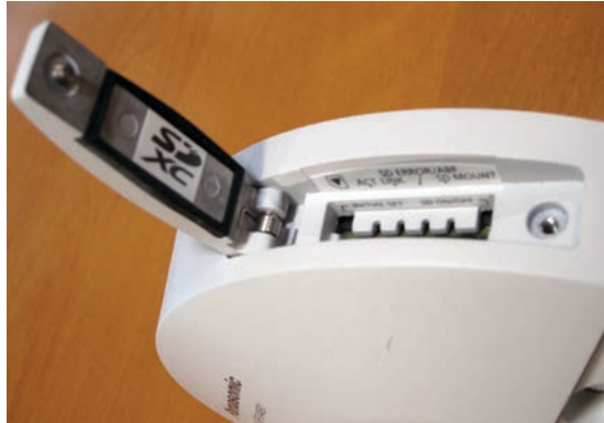
Although the evaluation camera was labeled "sample," the hope is it is identical to production versions. The WV-SFV481 has a built-in SD card slot under a trap door on the side of the camera that accepts cards up to 64GB.
