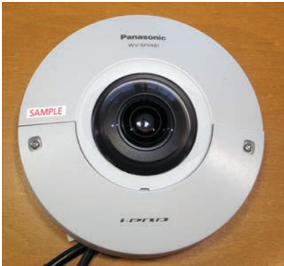
Although the evaluation camera was labeled "sample," the hope is it is identical to production versions. The WV-SFV481 has a built-in SD card slot under a trap door on the side of the camera that accepts cards up to 64GB.
