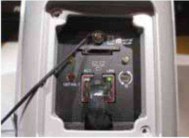
A small trap door on the assembly base provides access to the camera connection, micro SD card slot and setup buttons.
