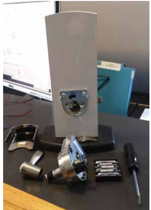
The SmartCode electronic lever's battery pack slides in/out easily and is stamped on the top “Door” with an arrow on either side of the stamp pointing to the side the door should be on. This product is easy to install and program, aesthetically pleasing and solidly built.
