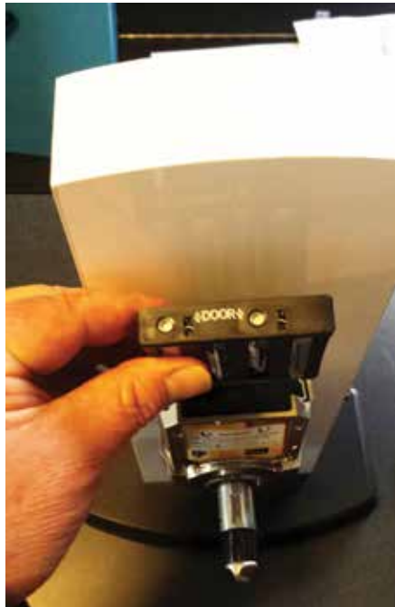
The SmartCode electronic lever's battery pack slides in/out easily and is stamped on the top “Door” with an arrow on either side of the stamp pointing to the side the door should be on. This product is easy to install and program, aesthetically pleasing and solidly built.
