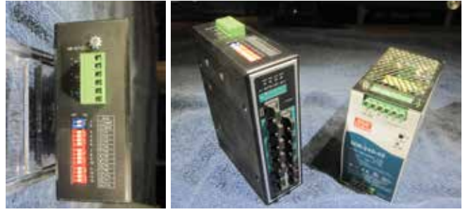
DIP switch configuration of the TI-PG1284i’s alarm outputs ( left ) makes setting up failure notification a breeze. The separate power supply ( right ) allows for redundant power where needed.
